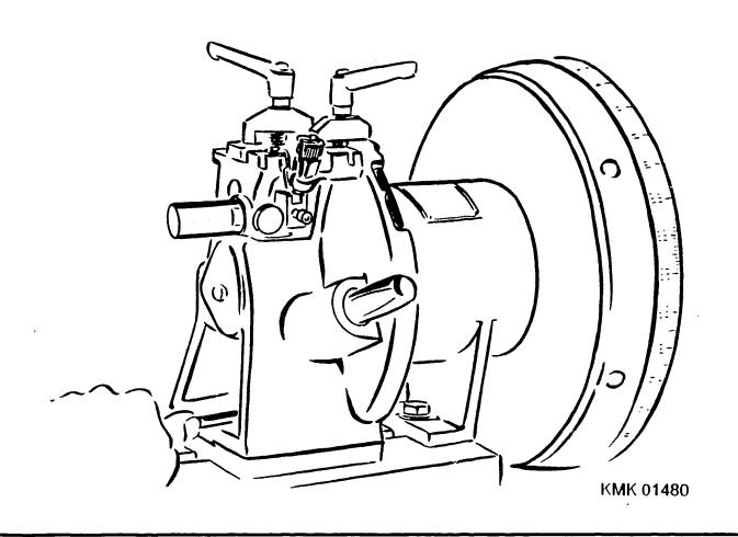
Attach dial-indicator 1 680 390 003 holder and insert control-rod-travel 1 687 233 015 dial indicator with screwed-in magnet. 1 686 540 013
